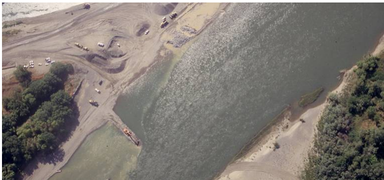
“Gradient Restoration Facility” on the Sacramento River, ca 1999. Structure across the channel to raise level for diversion
