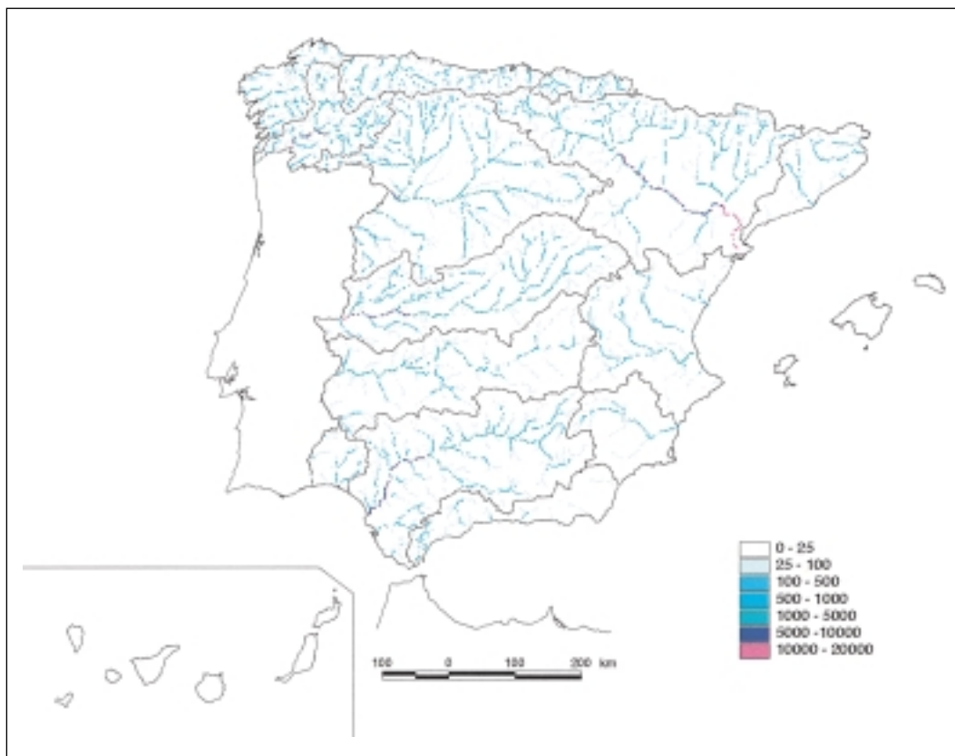
Figure 94. Map of total annual average cumulative flow (hm 3 /year) in the period 1940/41 - 1995/96.
