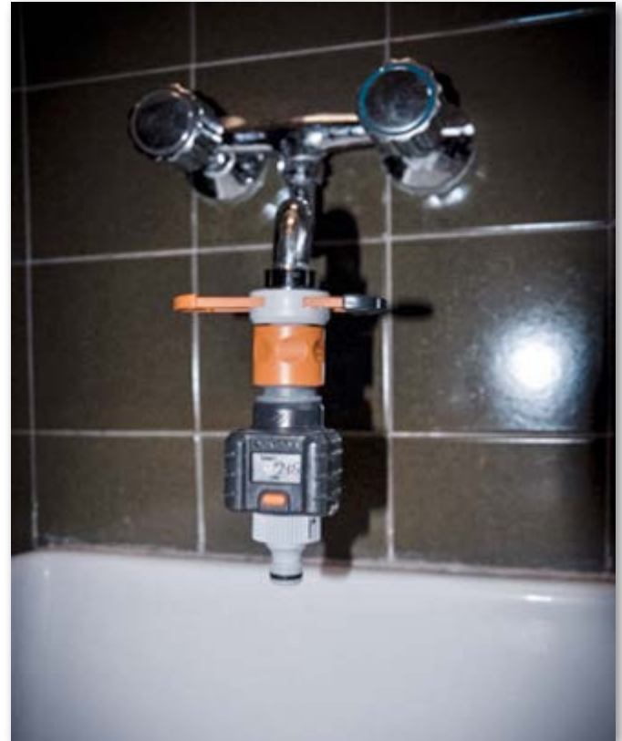
Litre counter to the school taps for measuring students water consumption. Chiara Dionigi, Consorzio abn.
