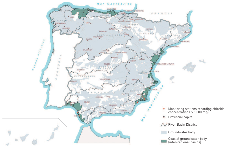
STATIONS RECORDING CHLORIDE CONCENTRATIONS ABOVE 1,000 mg/l (2005)
