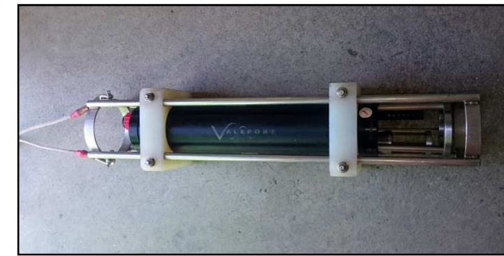
Figura 6 Sonda Valeport, Monitor SVP
