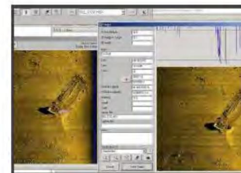
HYPACK® supports collection, targeting and mosaicking for both analog and digital side scans. It's a standard feature!
